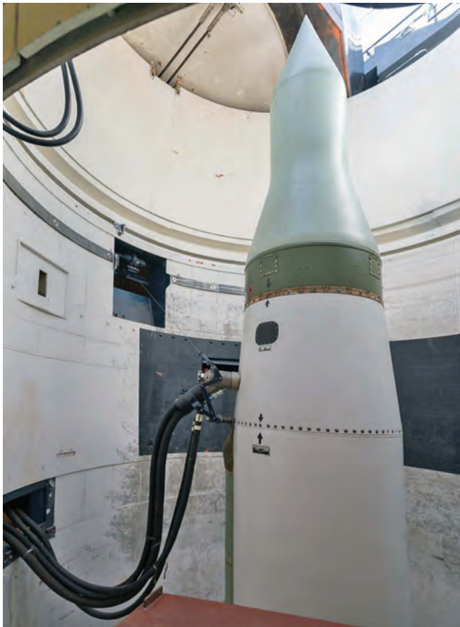
Minuteman II ICBM showing the re-entry vehicle at the top which would have contained the 1.2Megaton Thermonuclear warhead. The cable on the left is the electrical umbilical for the guidance system. Photo Chris Howells
